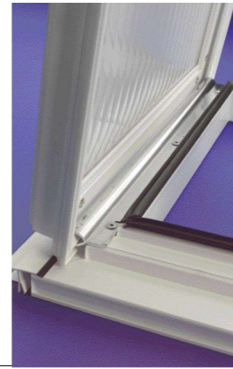
Full width hinge giving improved weather resistance
